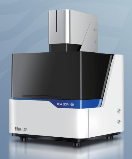
The TCA 3DP-160 employs infrared thermography-based non-contact thermometry integrated with 3D heat transfer inverse parameter identification methodology. Specifically designed for multilaminate composite structures with inherent anisotropic thermal conductivity (e.g., pouch-type lithium-ion battery cells, CFRP laminates), this system enables in-situ determination of both in-plane and through-plane thermal conductivities through full-field temperature mapping.
